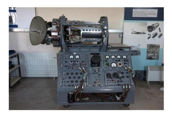
Typical 2<sup>nd</sup> line radar bay scene with the Lightning's Ferranti AI-23, removed from its 'bullet', fitted to a cradle and mounted on a test bed, the cradle allowing the radar to be rotated for access.
